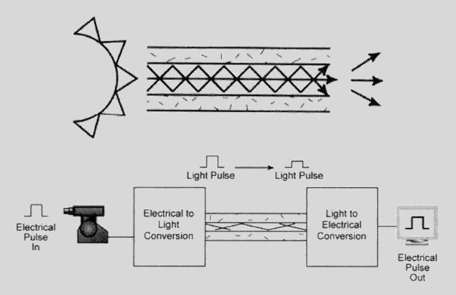
Fiber optic cable functions as a "light guide," guiding the light introduced at one end of the cable through to the other end. The light source can either be a light-emitting diode (LED)) or a laser.
