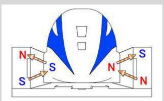
Additional guidance coils are sometimes used but since the current in the coils depends on the position of the magnets on the train, any displacements are often self-correcting. If you understand Faraday's Law you may be asking to yourself, won't there be no current in the coils when the train is not moving? The answer is yes and because of this a minimum speed is required to get the train off the ground. At low speeds the train is equipped with wheels.
