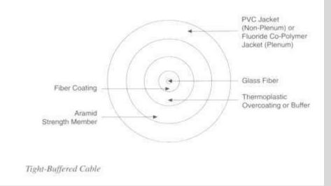
The use of fiber-optics was generally not available until 1970 when Corning Glass Works was able to produce a fiber with a loss of 20 dB/km. It was recognized that optical fiber would be feasible for telecommunication transmission only if glass could be developed so pure that attenuation would be 20dB/km or less.
