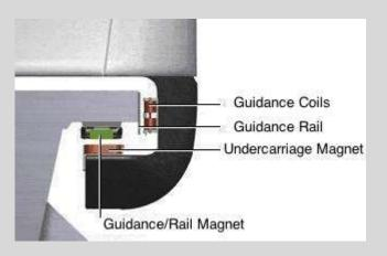
The figure shows that if the magnet on the guidance track is attracted to the magnet on the undercarriage, the train will levitate off the ground. It should be noted that no contact between the magnets is made since the strength of the attraction is only enough to get the train off the ground.
